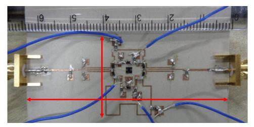
This filter will be measured to be 6.3 cm wide and (approximately) 2.5 cm long, for a total size of 15.75 cm<sup>2</sup>. Red arrows have been added to show the measurements.
