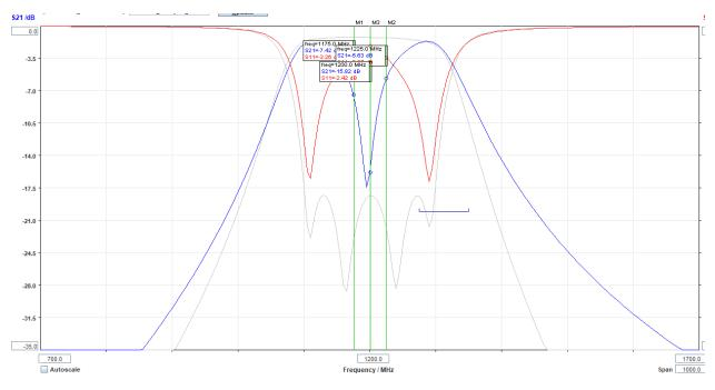
At 1.175, 1.2, and 1.225, the attenuation is 7.4, 15.8, and 5.6 dB. These measurements provide a positive point total of 28.8.
