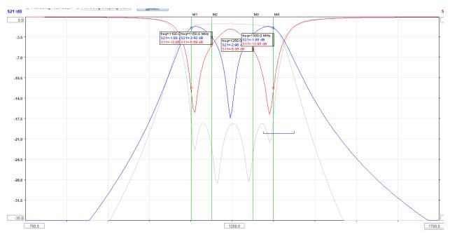
At 1.1, 1.15, 1.25, and 1.3 GHz, the attenuation is 1.9, 3.4, 3.0, and 1.9 dB, respectively. These measurements provide a negative point total of -10.2. The entire point total for scenario 3 is 28.8 - 10.2 = 18.6.
