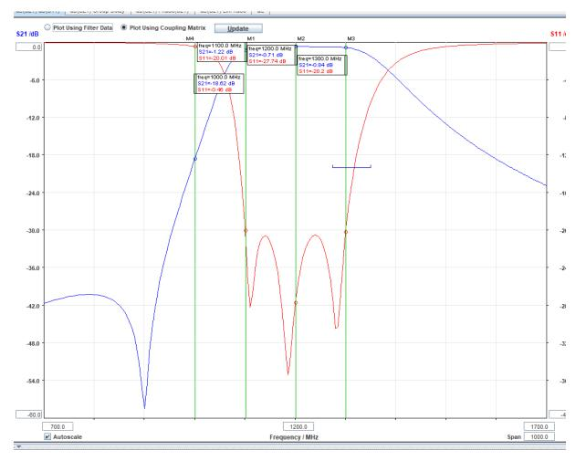
The insertion loss is measured at 1.0, 1.1, 1.2, and 1.3 GHz as 18.6, 1.2, 0.7, and 0.8 dB, respectively. The score for scenario 1 will be computed as 18.6 - 1.2 - 0.7 - 0.8 = 15.9. 15.9 is the score for this filter for scenario 1.
