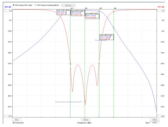
The insertion loss will be measured at 1.1, 1.2, 1.3, and 1.4 GHz as 0.9, 0.7, 1.2, and 11.9 dB, respectively. The score for scenario 2 will be computed as 11.9 - 0.9 - 0.7 - 1.2 = 9.1. 9.1 is the score for this filter for scenario 2.
