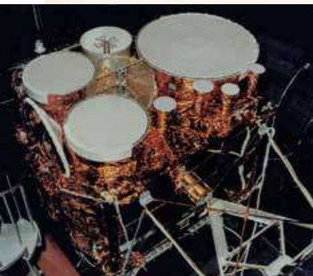
DSCS III Satellite, launched in 1982, in the thermal test facility at GE Aerospace, Valley Forge, PA. Photo provided by Mr. Herb Thal.
