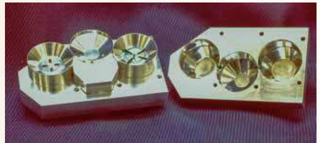
6 Pole, elliptic function TE011 mode filter with shaped cavities for mode control and increased unloaded Q, having a 40 MHz passband at 11725 MHz with two S21 nulls on each side and Q_u=20000 . (Circa 1978)
