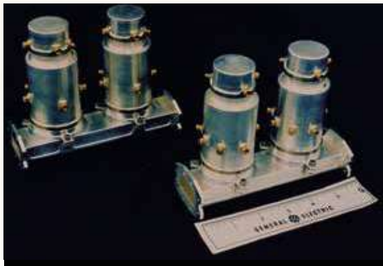
Hybrid TE113/TE111 mode, 4 Pole, directionally coupled, band reject filters for low-loss, narrow band rejection at 8 GHz for DSCS III. (Circa 1977)
