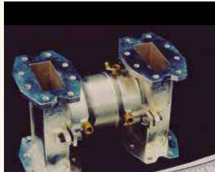
Directional Filter for Diplexing at 12 GHz for BSE TV Broadcast Satellite.
